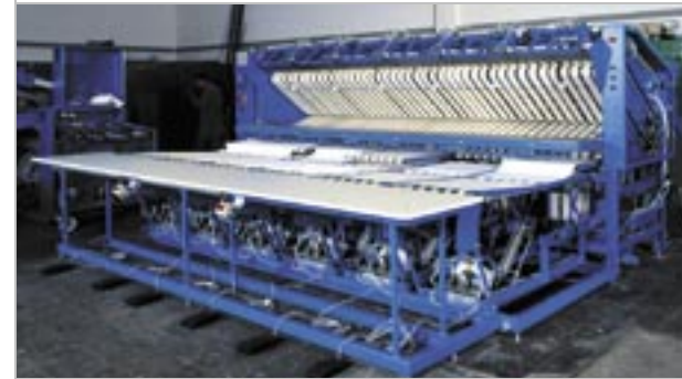
▲ ▼ 6-track folding machine for large laundry facilities: frequency inverter J7 allows variable speeds on the different track.
